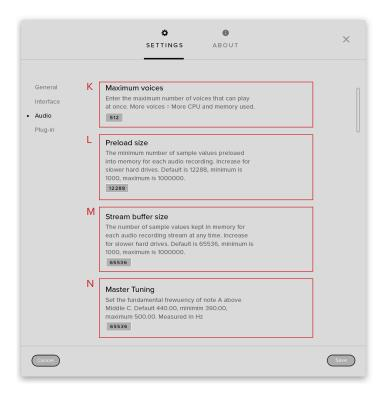
$\underline{\text{N. MASTER TUNING}}$  The default tuning (in Hz) of the A above middle C.
