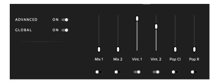
You can tell which are enabled by looking at the active switches below each signal.
